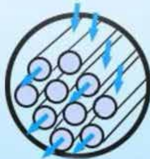
External Pressure No Clogging Issue, All Substances are remaining outside.
